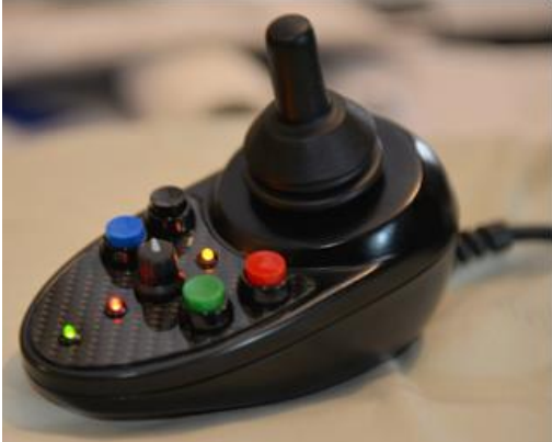
Custom built Hall affect pod using APEM Joystick.
